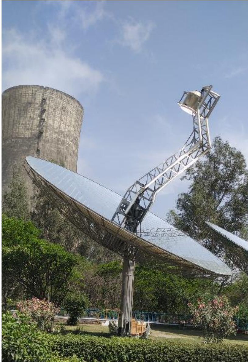
M95 Paraboloid Dish Concentrator: Peak Rating 40,000 kcals/hr
