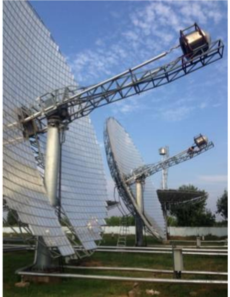
M95 Paraboloid Dish Concentrator: Peak Rating 40,000 kcals/hr
